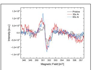
**Fig. 1**. ESR spectra of pristine and Ar<sup>+</sup>-treated SiO<sub>2</sub> thin films following 30 s and 60 s plasma exposure.
